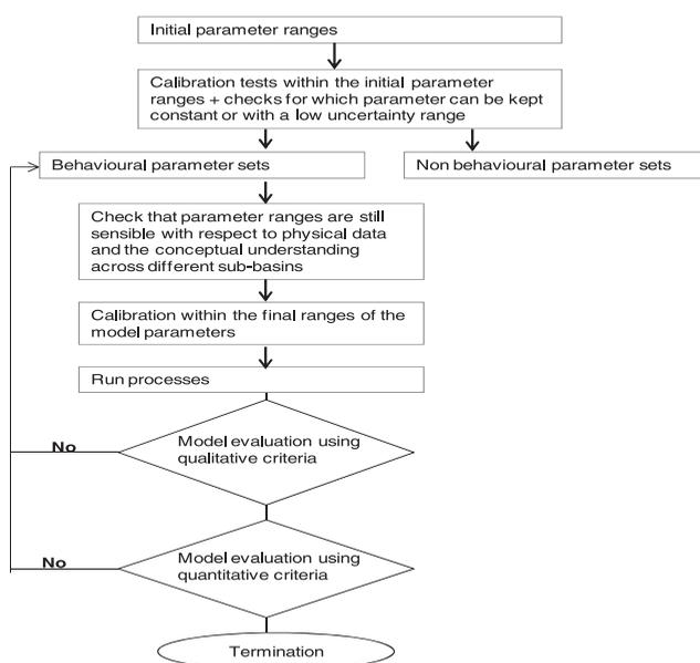
**Figure 4.** Procedures used for the GW-PITMAN model parameters estimation calibration in the Congo Basin.
